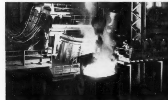
TOUR HIGHLIGHT will be visit to Bethlehem Steel Company's West Seattle electric-arc furnace plant; two new furnaces were installed in 1958. This tap is more than 100 tons.
